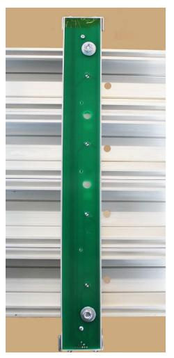
Slide the timer over the end of the track with the sensor bar beneath the track. Place the timer over the bolts installed in the previous step using the **timer's** track mounting holes (holes shown in picture on previous page). Then place a washer over each bolt and secure the timer with an additional nut on each bolt. **Finger tighten only. Do not over tighten.**
